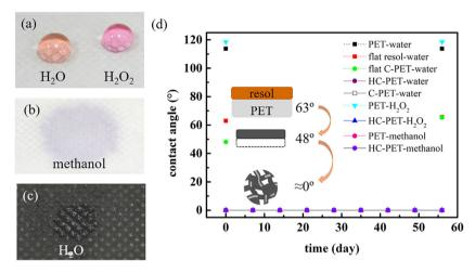
Figure 3. a) Water and  $H_2O_2$  liquid drops and b) methanol on the pristine PET; c) spread water drop on HC-PET; d) the CAs of different liquids on various samples in ambient condition.
