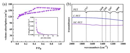
Figure 2. a)  $N_2$  adsorption-desorption isotherms of the HC-PET sheet; b) FT-IR data of PET, C-PET, and HC-PET fabrics.
