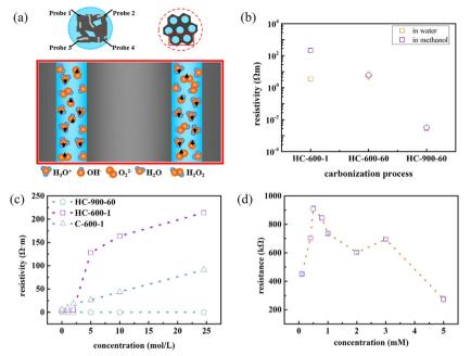
**Figure 5.** a) The scheme for liquid concentration detection; b) HC-PET sheets produced from different carbonization processes for water or methanol; c) resistivity changes of different porous materials in methanol solutions with different concentration; d) resistivity changes of HC-600-1 in  $H_2O_2$  solutions with different concentration.
