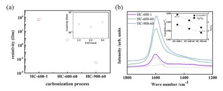
**Figure 4.** a) Resistivity of HC-PETs produced by different carbonization process, insert showed resistivity of HC-900-60 samples with different F127/resol ratios; b) Raman spectra of HC-PETs produced by different carbonization process, insert showed G peak position and  $I_D/I_G$  information.
