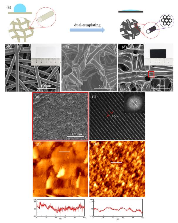
**Figure 1.** a) Scheme for comparison in structure between pristine PET and HC-PET fabrics; SEM images of b) pristine PET, c) C-PET sheet and d) HC-PET; e) locally magnified HC-PET fiber over a large domain; f) TEM and the corresponding fast Fourier transform (FFT) image; AFM profiles of g) C-PET, and h) HC-PET.
